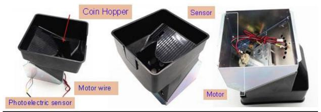
(On the picture, has the motor and sensor)
