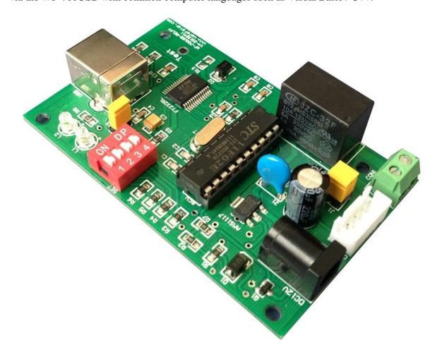
For USB version,that has a USB to RS232 chip on board to convert the RS232 to USB and build a virtual RS232 port in the PC. And user firstly need to install a driver in the PC for USB / RS232 chip. And the USB chip FT232RL driver download address:
