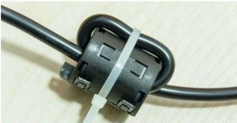
Put the DC12V power supply cable two or three times around the magnetic ring
