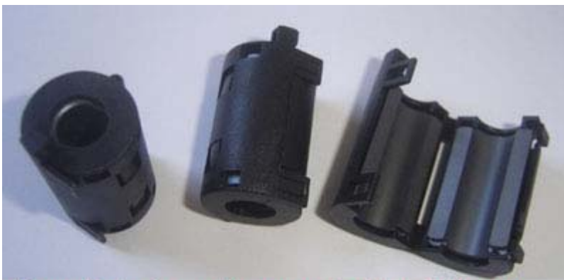
Magnetic ring is used to prevent motor interference
