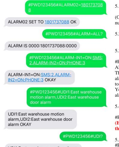
UDI1:East warehouse motion alarm, UDI2:East warehouse door alarm
