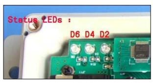
There are three LED: D2 D4 D6 on the board. That is used to show the working status of the device. D6 is used to show the GSM Module working status, D4 is used to show the MCU controller working status, D2 is used to show the Relay status, also when the relay is off, if incoming a SMS message,D2 will flash quicly to show the incoming message and also following
